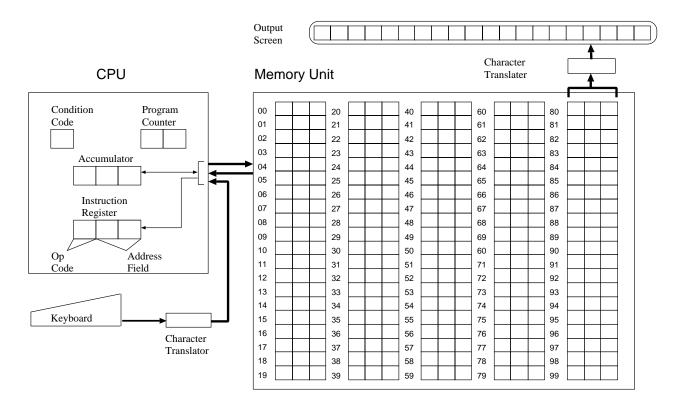
Figure 2.1: Itty Bitty Machine Architecture
