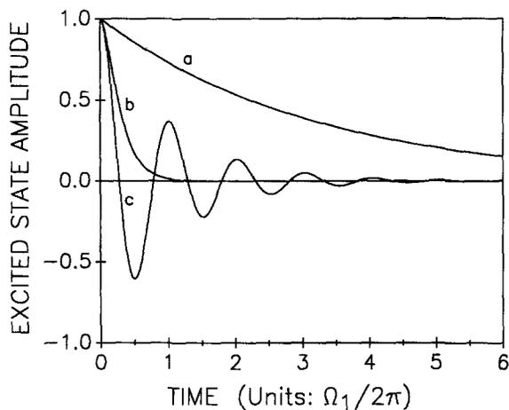
Fig. 5. Single atom in a single mode, damped cavity: Amplitude for the system to be in the state  $|e;0;\emptyset\rangle$  (excited atom, no photon, no wall excitations) as a function of time. This is a plot of Eq. (36) in the text. In curve "a" the atom-field oscillations are overdamped ( $\gamma_{\text{cav}}/\Omega_1=40$ ), in "b" the oscillations are critically damped ( $\Omega_{\text{cav}}/\Omega_1=4$ ), and in "c" the oscillations are underdamped ( $\gamma_{\text{cav}}/\Omega_1=0.63$ ).
