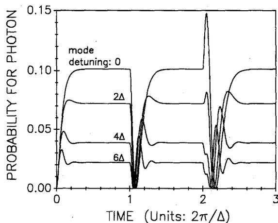
Fig. 3. Single atom in center of multimode cavity: Probabilities for the system to be in representative states  $|g; n\rangle$  (ground state atom, one photon in mode with detuning  $n\Delta$ ) as a function of time. The probabilities initially grow with time and then reach a relatively constant value until the first revival of the atomic excitation at time  $T_{\text{recurrence}} = 2\pi/\Delta$ . Atomic parameters are the same as in Fig. 1.
