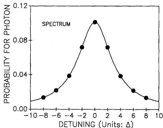
Fig. 4. Single atom at center of multimode cavity: Spectrum of photon probabilities at "long" times. The points are taken from the data plotted in Fig. 3 at time  $t=6/\Delta$ . This time is well after the atom has decayed, but before the first revival at time  $T_{\text{recurrence}} = 2\pi/\Delta$ . The line is a Lorentzian curve with a full width at half-maximum equal to  $2\gamma$ .
