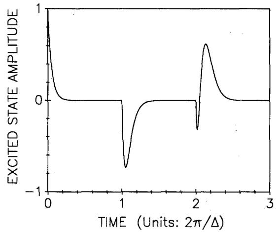
Fig. 1. Single atom at center of multimode cavity: Amplitude for the system to be found in the state  $|e; \emptyset\rangle$  (excited atom and no photon) as a function of time. This is a plot of Eq. (19) in the text. Note the initial exponential decay and the subsequent revivals. The atom-field coupling strength,  $\Omega$ , for this plot is set equal to the mode frequency spacing,  $\Delta$ .
