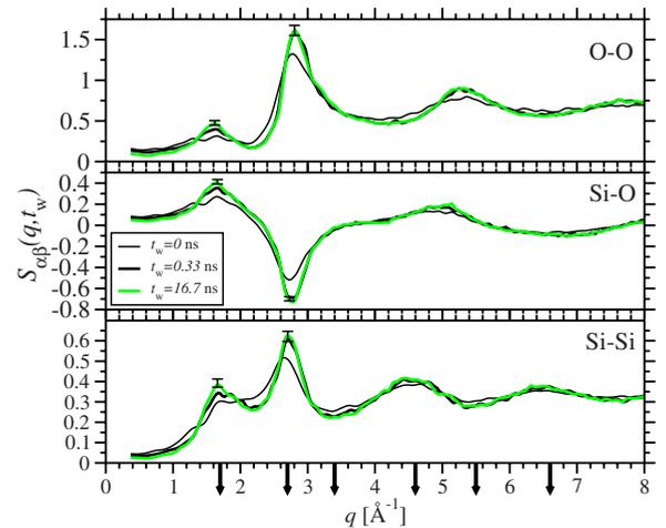
FIG. 3. (Color online) Partial structure factors  $S_{\alpha\beta}(q, t_w)$  as defined in Eq. (2) for the temperature quench from  $T_i=5000$  K to  $T_f=2500$  K. Indicated with arrows are the wave vectors  $q$ , which have been used to determine  $C_q(t_w, t_w + t)$  as defined in Eq. (3).
