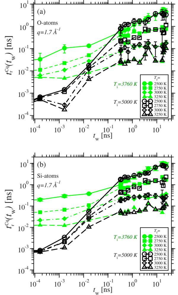
FIG. 7. (Color online) Decay time  $t_r^{Cq}$  for  $q = 1.7 \text{ \AA}^{-1}$  and (a) O-atoms and (b) Si-atoms. Green (gray) is used for  $T_i = 3760$  K and black for  $T_i = 5000$  K. Symbol shape indicates  $T_f$  as given in the legend. Error bars are given exemplarily for  $(T_i = 3760 \text{ K}, T_f = 2500 \text{ K})$ ,  $(T_i = 5000 \text{ K}, T_f = 2500 \text{ K})$ , and  $(T_i = 5000 \text{ K}, T_f = 3000 \text{ K})$ .
