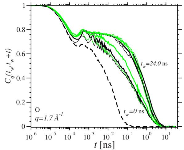
FIG. 6. (Color online)  $C_q(t_w, t_w + t)$  for the quench  $T_i=3760$  K to  $T_f=3000$  K. Waiting times and corresponding line styles are the same as in Fig. 4. Error bars are of the same order as indicated in Fig. 4. The thick dashed line corresponds to  $C_q(t_w, t_w + t) = F_s(q, t)$  at 3760 K.
