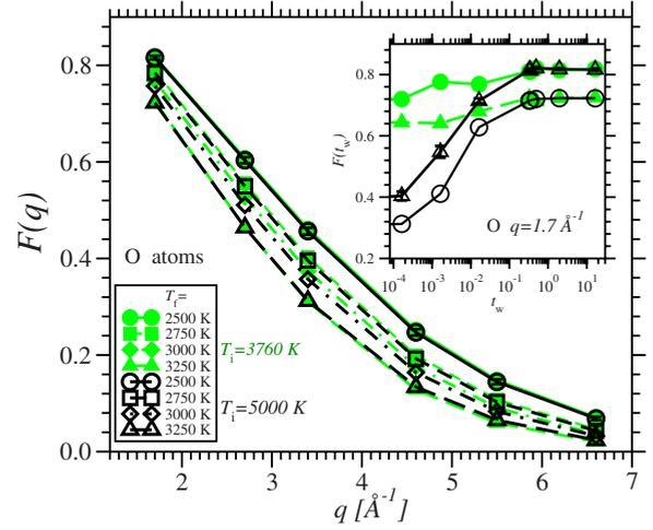
FIG. 5. (Color online) Plateau height,  $F$ , as defined in the text, as a function of wave vector  $q(t_w=16.67$  ns) and in the inset as a function of  $t_w$  ( $q=1.7 \text{ \AA}^{-1}$ ). Error bars are of the same size as symbols as indicated exemplary for  $T_i=5000$  K and  $T_f=2500$  K.
