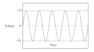
(The *peak-to-peak* amplitude is  $2V_0$ , and the *RMS* amplitude is  $V_0/\sqrt{2}$ .)
