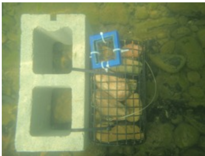
Figure 2. Rock basket sampler in the West Branch Susquehanna River. Benthic macroinvertebrates colonize rocks in the samplers over 6 weeks and can provide a standardized method for comparing communities across sites. [Photo: Matt McTammany]
