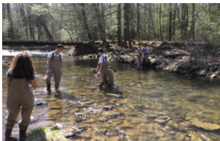
Civil Engineering students in Jessica Newlin's River Engineering (CENG 422) class measure stream cross-sections, discharge, and the distribution of sediment size on the channel bottom. [Photo by Sean Reese]
