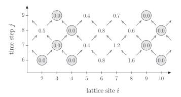
FIG. 1. An illustration of the parallel update in d=1. All particles occupy even (odd) numbered sites at even (odd) numbered time steps. The circles represent A particles, with an  $A+A \rightarrow A$  reaction occurring at site i=3 and time step j=7. The numbers represent the means of the Poisson distribution of B particles, which are updated according the rules in Eqs. (8) and (9), with p'=1.
