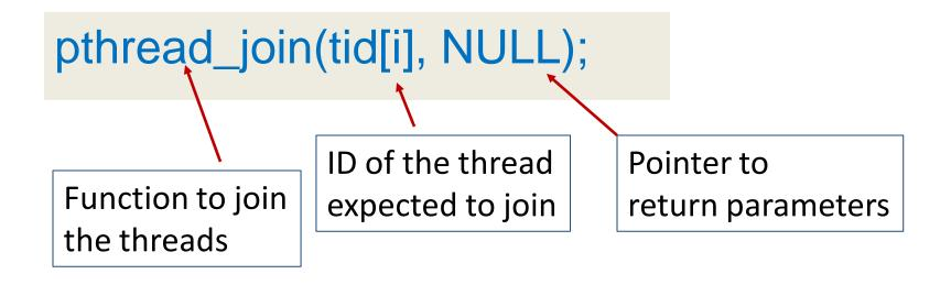
The second parameter is of the type void **\*\***ptr, which is an address to a pointer (pointer to a pointer). If it is used, usually it returns the exit status of the thread.
