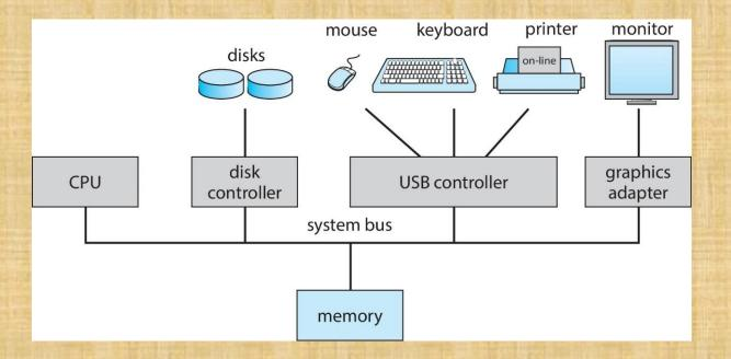
The blocks shown are hardware components. Software runs on these components.
