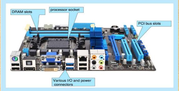
This board is a fully-functioning computer, once its slots are populated. It consists of a processor socket containing a CPU, DRAM sockets, PCIe bus slots, and I/O connectors of various types. Even the lowest-cost general-purpose CPU contains multiple cores. Some motherboards contain multiple processor sockets. More advanced computers allow more than one system board, creating NUMA systems.
