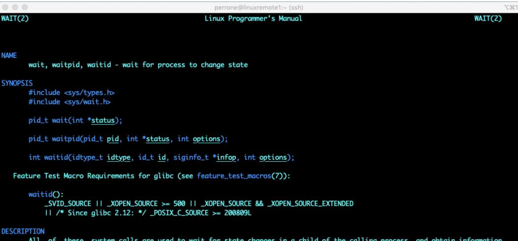
All of these system calls are used to wait for state changes in a child of the calling process, and obtain information about the child whose state has changed. A state change is considered to be: the child terminated; the child was stopped by a signal; or the child was resumed by a signal. In the case of a terminated child, performing a wait allows the sys-Manual page wait(2) line 1 (press h for help or q to quit)
