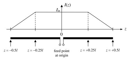
**2.** For the antenna in the previous problem, derive an expression for the radiation resistance as a function of the length l. Obtain a numerical value for  $l = 0.02\lambda$ , and compare it to the radiation resistance of a standard short dipole (with a triangular current distribution) and that of a Hertzian dipole (uniform distribution) of the same length.
