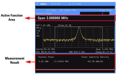
Avg Number On Off Specifies the number of measurement averages used when calculating the measurement result with Avg Number (On). The range of the number is from 1 to 1000. Use the knob, the arrow keys or the numeric keypad to set the number. The average will be displayed at the end of each sweep. Selecting Off disables measurement averaging.
