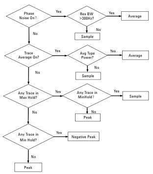
When the detector sets to Auto, Pressing  $\mathbb{E}_{Mn}$  > Average (On) changes the detector. The Auto choice depends on marker functions, trace functions, and the trace averaging function. If a marker function or measurement is running, the Auto choice of detector is either Average or Sample. When one of the detectors (such as Average) is manually selected instead of Auto, that detector is used without regard to other analyzer settings.
