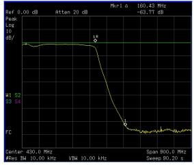
Figure 19 Measure the Rejection Range
