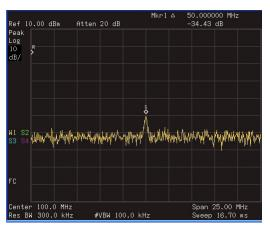
Figure 3 Delta Marker with Reference Signal Off-Screen
