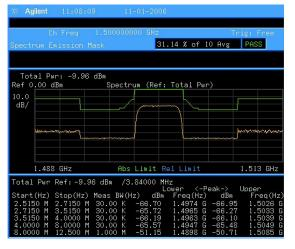
Avg NumberSet Avg Number to On to specify the number of measurement<br/>averages used when calculating the measurement result. The<br/>average will be displayed at the end of each sweep. Setting<br/>Avg Number to Off disables measurement averaging.<br/>Key access: MeasMeas> More > Spectrum Emission Mask
