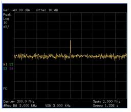
A "#" mark appears next to the Res BW annotation in the lower left corner of the screen, indicating that the resolution bandwidth is uncoupled.
