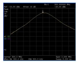
**4** Change the resolution bandwidth (RBW) to 100 kHz so that the RBW setting is less than or equal to the frequency separation of the two signals:
