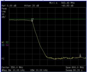
Figure 21 Minimum Stop Band Attenuation
