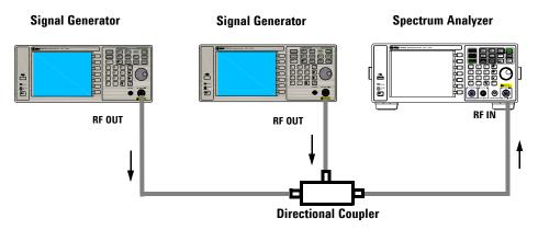
Figure 4 Setup for obtaining two signals
