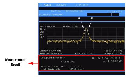
Figure 29 Occupied Bandwidth Measurement
