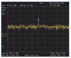
Note that increasing the attenuation moves the noise floor closer to the signal level.
