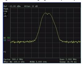
For fastest measurement times, use the widest possible resolution bandwidth. Under factory preset conditions, the resolution bandwidth is coupled to the span.
