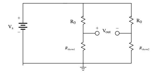
In this bridge, the output voltage V<sub>out</sub> is now a difference between the two sides of the bridge.
