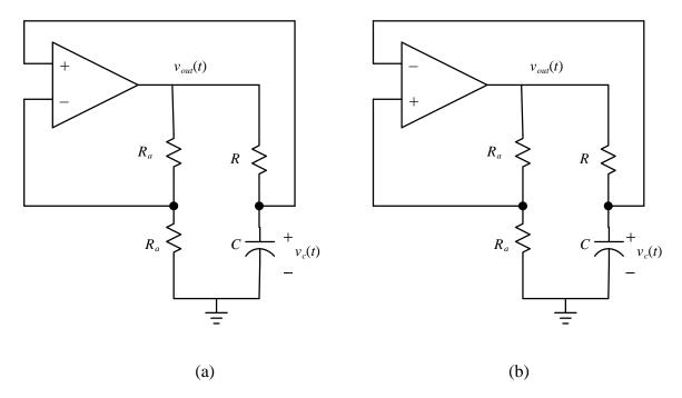
**Pre–Lab Question:** What does circuit (a) do? Will it oscillate? Does it operate differently than circuit (b)?
