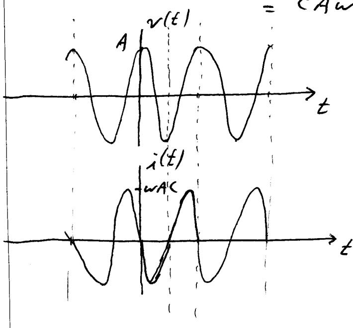
Current is scaled in amplitude by factor  $\omega C$ , and shifted in phase by  $90^\circ$ , relative to voltage.
