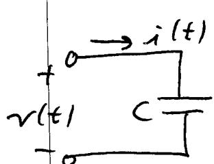
$$\begin{aligned} i(t) &= C \frac{dv}{dt} \\ &= C \cdot \frac{d}{dt} A \cos \omega t \\ &= -CA\omega \sin \omega t \\ &= CA\omega \cos[\omega t + 90^\circ] \end{aligned}$$
