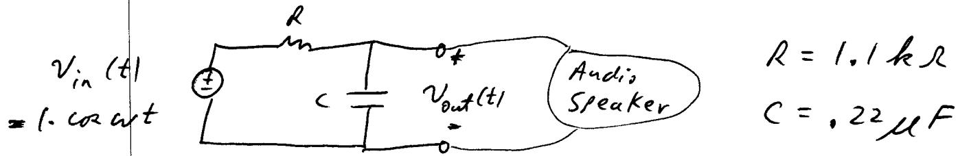
Vary  $\omega$ , the frequency of input sine wave.
