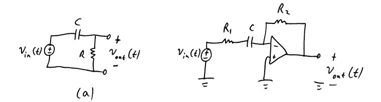
5. Classify each of the following filters as low-pass, high-pass, or band-pass. You can do this by looking at each filter as a voltage divider, and determining the behavior of each impedance in the circuit for low frequencies, middle frequencies, and high frequencies. Alternatively, you can write the equation for the frequency response and study its behavior as the frequency varies.
