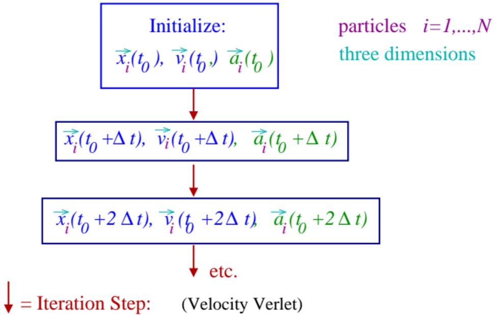
$$\begin{aligned}\vec{x}_i(t+\Delta t) &= \vec{x}_i(t) + \vec{v}_i(t)\Delta t + \vec{a}_i(t)(\Delta t)^2/2 \\ \vec{v}_i(t+\Delta t) &= \vec{v}_i(t) + (\vec{a}_i(t) + \vec{a}_i(t+\Delta t)) \Delta t/2 \\ \vec{a}_i(t) &= \vec{F}_i(t)/m_i = -\nabla_{\vec{r}_i} U(t)/m_i\end{aligned}$$
