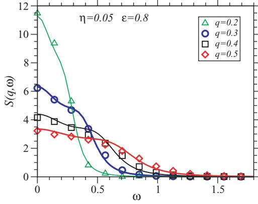
FIG. 11. (Color online) Dynamic structure factor  $S(q, \omega)$  for  $\eta = 0.05, \varepsilon = 0.8$ , and  $q = 0.2 - 0.5$ . Symbols indicate simulation results obtained via Fourier transform of  $F(q, t)$ , and lines indicate fits with Eq. (33).
