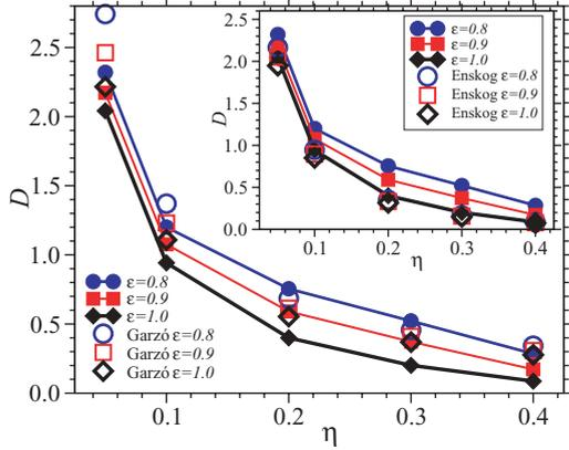
FIG. 5. (Color online) Self-diffusion constant  $D$  as a function of volume fraction  $\eta$ . Filled symbols, with lines to guide the eye, were obtained via linear fits to the mean square displacement for large times. Garzó results correspond to Eq. (2.10) of Ref. [28], and the Enskog result corresponds to Eq. (5) of Ref. [21].
