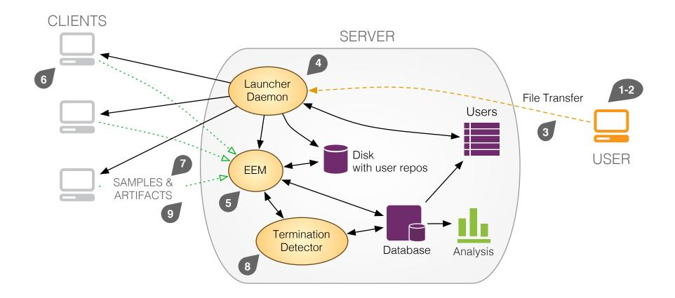
6) Clients detect number of cores and spawn one SC for each. SCs request a design point and spawn ns-3 execution: samples generated sent to EEM.
