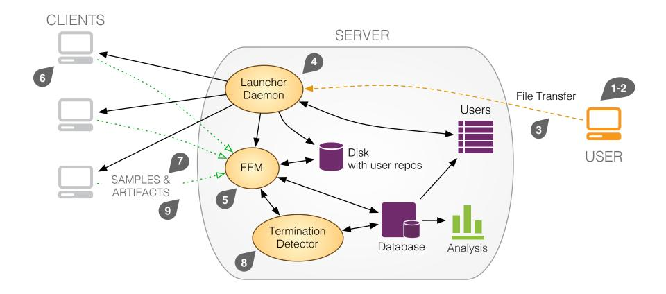
5) Launcher daemon starts: EEM with NEDL file; termination detector process. EEM computes design points and waits for requests.
