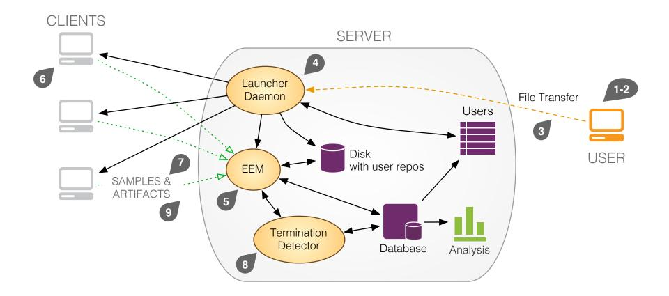
3) ns-3 installation archived; credentials verified with server; bundle transferred to user compartment in server under unique experiment id.
