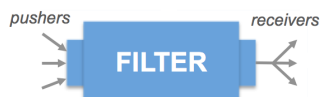
Figure 2. The Filter module modifies data in some way, receiving input from one-to-many Pushers, and outputting data to one-to-many Receivers.
