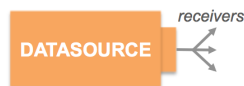
Figure 1. DataSources can represent any form of streaming input, outputting the raw data to one-to-many Receivers
