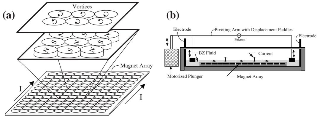
Fig. 2: (a) Exploded view of magnetohydrodynamic forcing. A  $40 \times 40$  array of magnets with alternating polarity sits below a fluid layer through which a current passes, producing an array of vortices. (b) Side view of apparatus. The fluid layer is 3 mm thick. A pair of displacement plungers slowly oscillates the fluid left-right across the vortex array; another set (not shown) oscillates the fluid horizontally in-out of the plane of the page.
