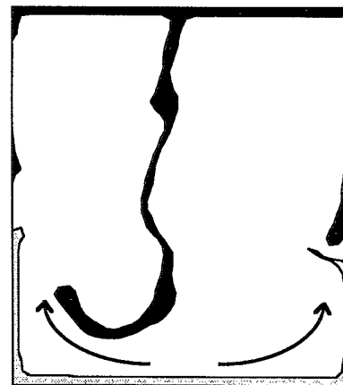
FIG. 6. Example of the dominant thermal features with single-vortex forcing. This sketch is based on liquid-crystal thermography. The secondary flow advects warm fluid (light shading) up along the side walls of the cell and creates a non-bursting lower boundary layer. Cool thermal plumes (dark shading) falling from the top are unopposed and frequently span the full height of the cell.
