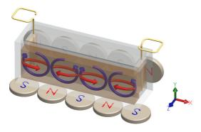
FIG. 1. Fluid cell, showing the magnetohydrodynamic forcing and the resulting flow formed from the superposition of a horizontal (red) and vertical (blue) chain of vortices. The fluid channel measures  $0.80 \times 8.0$  cm horizontally with a height of 1.9 cm.
