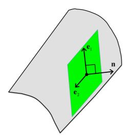
FIG. 6. A front element with normal vector  $\mathbf{n}$  and tangent vectors  $\mathbf{e}_1$  and  $\mathbf{e}_2$ .
