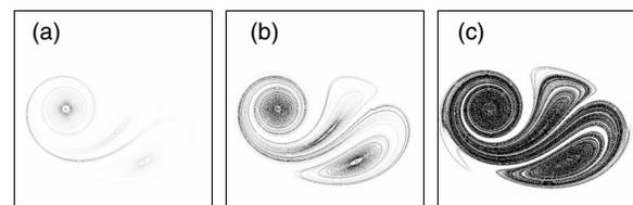
FIG. 4. Simulated maps of the mixing field after (a) 2.0, (b) 3.0, and (c) 5.0 oscillation periods;  $\mu = 0.52$ . The scaling of the intensity is the same for the three images and has been chosen to highlight the main features. The mixing field for one period of oscillation (not shown), corresponding to  $f = 0.010$  Hz, is relatively featureless when plotted with the same scaling factors as those shown here.
