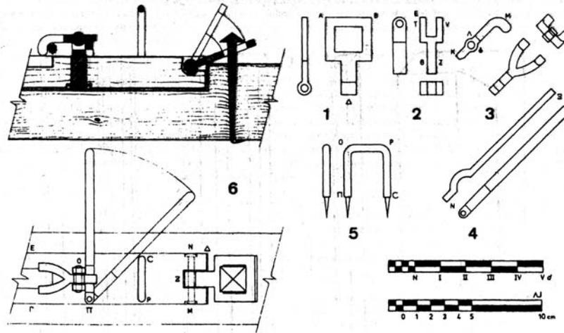
Fig. 3: 1. The 'handle'. 2. The fork. 3. The claw. 4. The trigger. 5. The pitirion. 6. Assembled trigger mechanism. Longitudinal section and plan.
