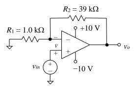
An expression for the closed-loop voltage gain  $v_o/v_{in}$  that accounts for the effect of the finite open-loop gain  $A_o$  is given by
