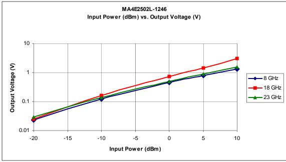
The MA4E2502L-1246 chip was evaluated in a detector circuit in which the Schottky diode terminates a 50 ohm transmission line on a duroid substrate. The chip was attached to the terminal of a 3.5mm connector and the output voltage was measured through a bias tee on a voltmeter. Matching was not attempted.
