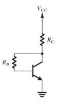
$$I_C \approx \frac{V_{CC} - V_{BE}}{\frac{R_B}{\beta} + R_C}$$
