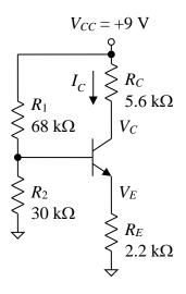
2. For the circuit considered in the previous problem, find the value of resistor  $R_C$  that would cause the BJT to operate right at the boundary of the saturation and active regions.
