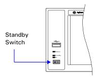
Pressing this front panel switch toggles power to the signal generator between on (green LED on) and standby (orange LED on). In standby mode, the signal generator is switched off, but the instrument is still connected to the line power. The rear panel line switch and the detachable power cord is the instrument disconnecting device. The front panel power switch, therefore, is not, and should not be used as a power switch.
