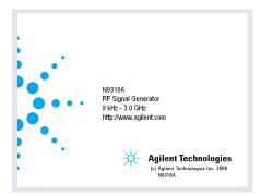
Self-initialization takes about 30 seconds, including self-test. If it detects an error, it reports an error message. The signal generator then defaults to a maximum frequency of 3 GHz and a minimum amplitude of -127 dBm, then the signal generator is ready for your current use. After power on, let the signal generator warm up for 45 minutes for stabilization.
