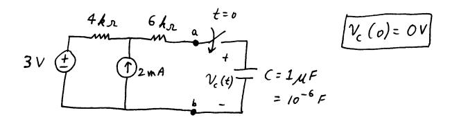
One way to solve this problem is to find the Thevenin equivalent circuit for the circuit to the left of terminals a and b. Then, you can consider the capacitor as the "load," and you can find  $v_c(t)$  by attaching the capacitor to the Thevenin equivalent circuit. If you use this approach, then remember you can use nodal analysis to help you solve for the open-circuit voltage and the short-circuit current.
