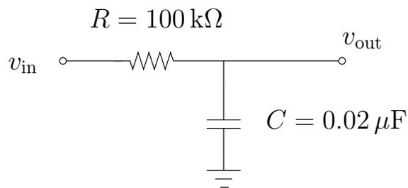
4. (20 pts) The input to the illustrated circuit is a sine-wave with angular frequency  $\omega$ . Derive a formula that gives the output voltage in terms of the input voltage and variables  $\omega$ ,  $R$ , and  $C$ . Does the output lead or lag the input? (There is more than one way to do this problem.)
