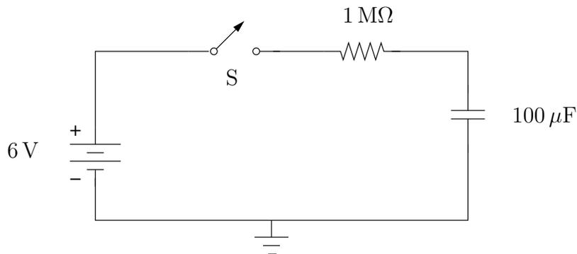
28. Prove that the 10% to 90% rise time for a  $RC$  low-pass filter is  $2.2RC$  for a perfect step-function input.
