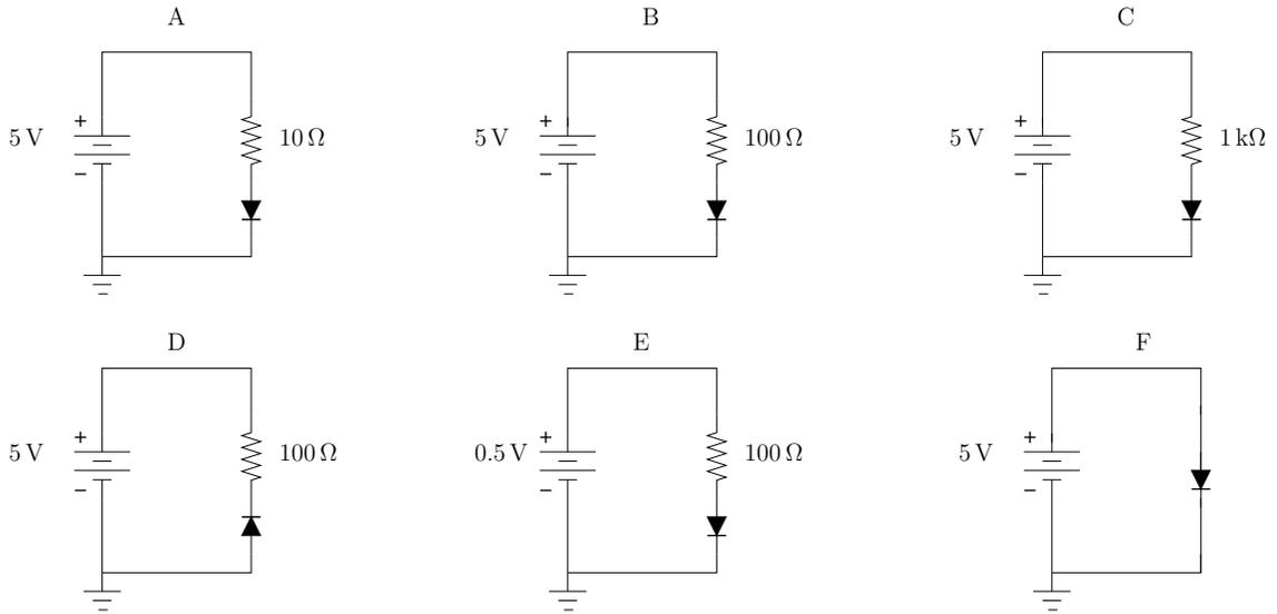
47. Repeat the previous problem for LEDs with a turn-on voltage of 2.5 V.
