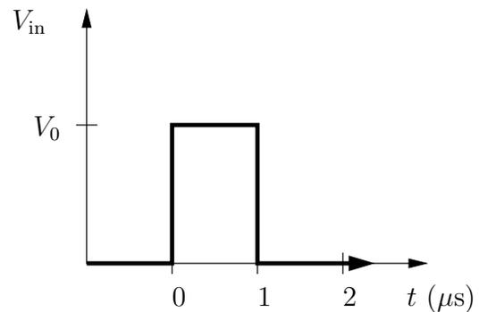
31. The graph below shows the input to the illustrated circuit. On the same graph sketch the output.
