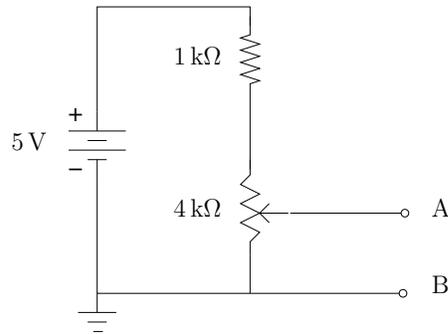
10. Calculate the voltage difference between points A and B. Which point is at a higher potential, A or B?
