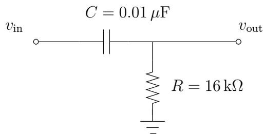
32. Calculate the capacitive reactance (i.e., magnitude of the impedance) in ohms of a  $0.01 \mu\text{F}$  capacitor at (a) 100 Hz, (b) 1 kHz, (c) 100 kHz, (d) 1 MHz.
