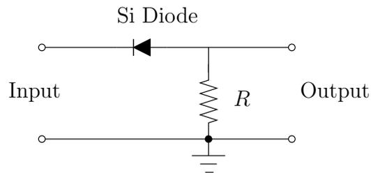
Sketch the voltage output waveform for the illustrated input.
