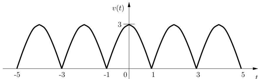
110. Fourier analyze the illustrated periodic rectified sine wave, i.e., determine expressions for the coefficients  $a_0$ ,  $a_n$ , and  $b_n$ , and for  $\omega$ , in the Fourier representation of the signal,
