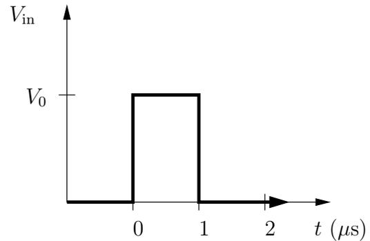
30. Sketch the approximate output from an  $RC$  differentiating circuit (i.e., an  $RC$  high-pass filter) with  $R = 10\text{ k}\Omega$  and  $C = 0.4\text{ nF}$  for the illustrated inputs. For the input on the left, make sure that your sketch of the output has an appropriate time scale indicated on the axis.
