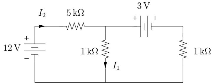
15. Calculate  $I_1$ ,  $I_2$ , and  $I_3$  in the illustrated circuit.
