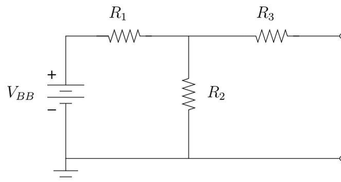
25. Calculate the Norton equivalent for the illustrated circuit at the indicated output terminals.
