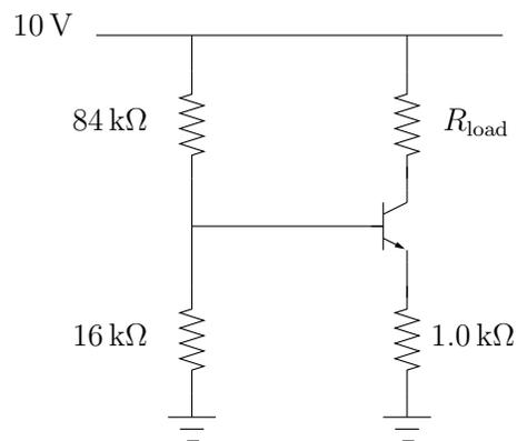
60. Consider the simple common-emitter amplifier discussed in class. (This is also part of the amplifier that some of you built in the optional part of the Introduction to Transistors Lab.) Consider as the input the voltage  $V_{in} = 1.59 + 0.33 \cos(\omega t)$ , i.e., a signal that oscillates between  $1.59 - 0.33 = 1.26 \text{ V}$  and  $1.59 + 0.33 = 1.92 \text{ V}$ .
