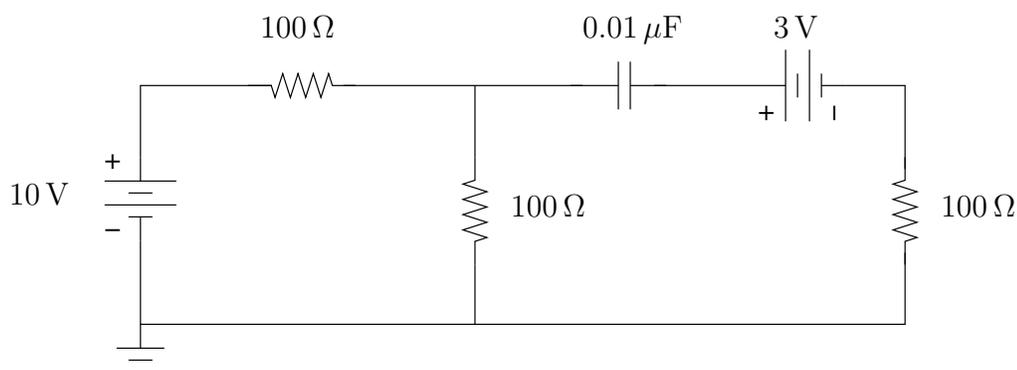
27. Consider the illustrated circuit that starts with the capacitor initially uncharged. The switch  $S$  is closed, and the capacitor begins to charge. What is the time interval between the time the capacitor is charged to 3 V and the time the capacitor is charged to 3.78 V?
