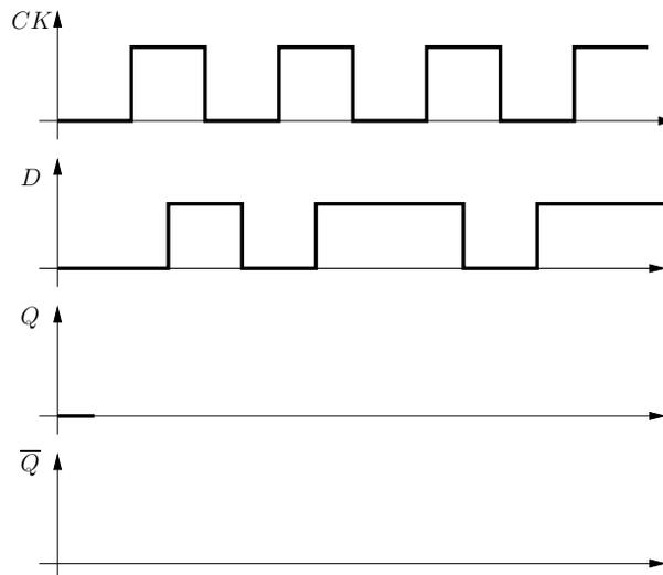
95. The illustrated circuit is made of positive edge-triggered type  $D$  flip-flops.
