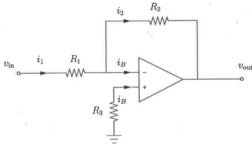
Determine the value of  $R_3$  that will cancel the offset, i.e., determine a value of  $R_3$  that will make the output
