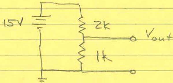
To find  $V_{th}$  measure the open-circuit voltage across the outputs. In other words, use a good voltmeter (high-resistance - draws no current).
