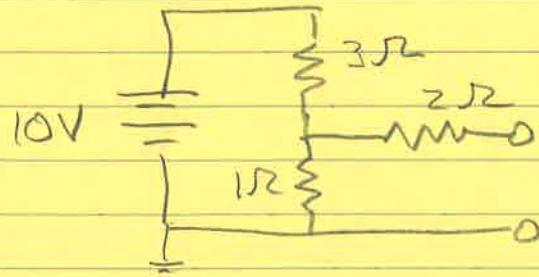
When the outputs are an open circuit no current flows through  $2\Omega$  resistor, so  $\Delta V_{2\Omega} = 0$ , and the measured  $V_{oc}$  is simply the voltage provided by  $3\Omega - 1\Omega$  voltage divider.
