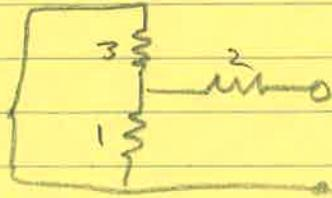
$\leftarrow$  Parallel combination of  $1\Omega + 3\Omega$  in series with  $2\Omega$
