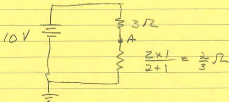
$$V_A = \frac{\frac{2}{3}}{3 + \frac{2}{3}} \times 10 \quad \leftarrow \text{voltage divider}$$
