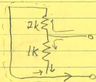
This is actually a parallel combination of the resistors.
