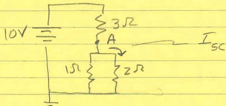
To find  $I_{sc}$  we need to know the voltage at A,  $V_A$ . To do this, first find the parallel combination of the  $1\Omega + 2\Omega$  resistors
